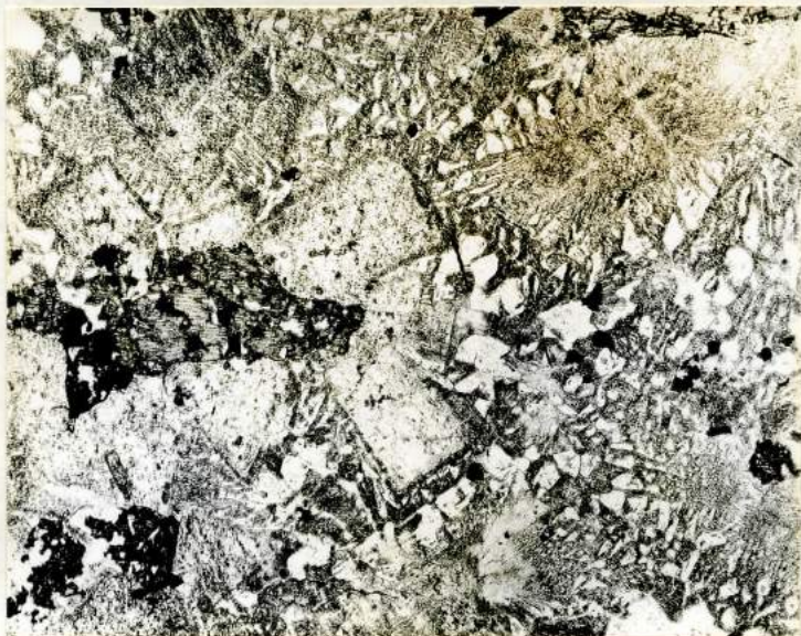
Fig.31. Photomicrograph of a typical granophyre (H304) from the Austurhorn intrusion. Phenocrysts of ferroaugite and euhedral plagioclase (with margins of turbid alkali feldspar) lie in a micrographic groundmass of quartz and alkali feldspar. X20. Ordinary light.
